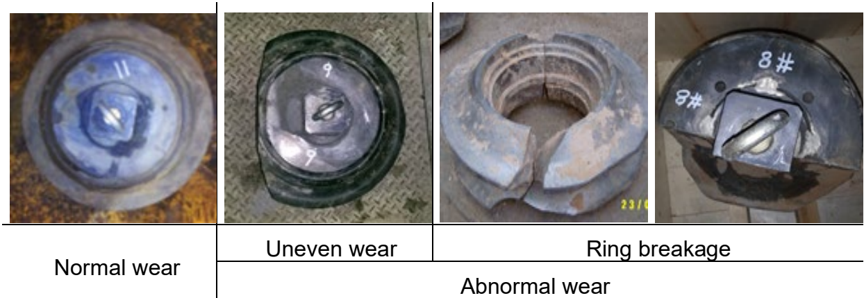
Fig. 3 Site-observed disc cutter wear at replacement
